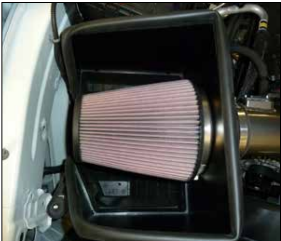
21. Install the K&N air filter onto the adapter and secure with the provided hose clamp.
