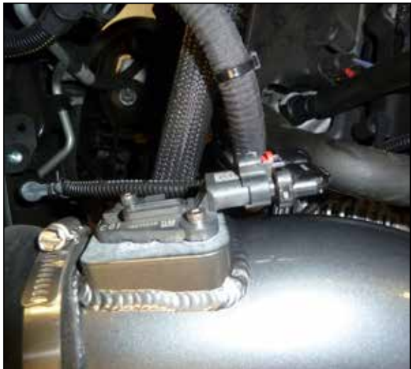
20. Reconnect the mass air sensor electrical connection.
