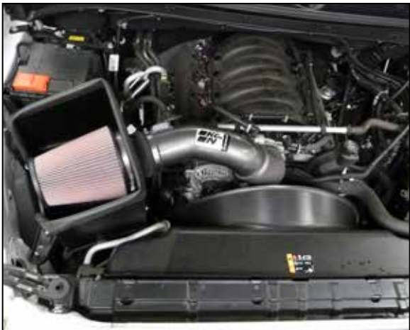
22. Reconnect the vehicle's negative battery cable. Double check to make sure everything is tight and properly positioned before starting the vehicle.
