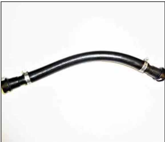
18. Assemble the CCV hose with the fittings, hose and clamps provided.
