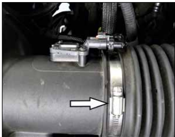
4. Loosen the hose clamp securing the intake hose to the air filter housing. Disconnect the mass air sensor electrical connection.
