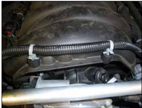
7. Disconnect the wiring harness from the intake manifold.
