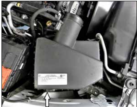
6. Loosen the seven screws that secure the upper air filter housing to the lower housing, then remove the upper housing and factory air filter.
