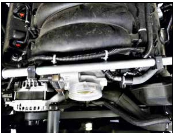
9. Secure the wiring harness and coolant pipe to the mounting bracket as shown.
