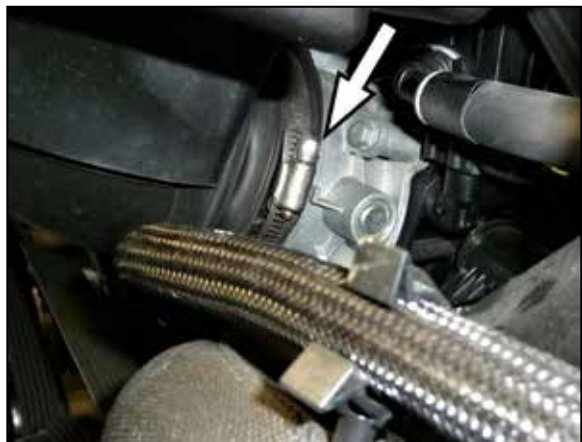
5. Loosen the hose clamp that secures the intake plenum to the throttle body. Remove the intake plenum from the vehicle.
