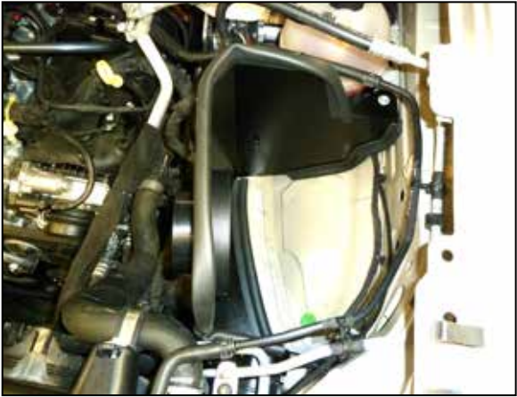
13. Install the heatshield assembly into the vehicle and position to OEM air box locations. Secure using OEM bolt.
