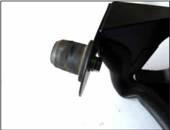
12. On the front side tab of heatshield, install the threaded boss with hardware and secure and tighten. Remove the factory rubber isolator from the OEM air box and attach to the threaded boss like image shown.
