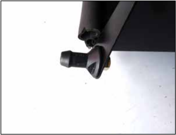
11. Attach the plastic air box mount with hardware provided to the bottom of the heatshield. Secure and tighten.
