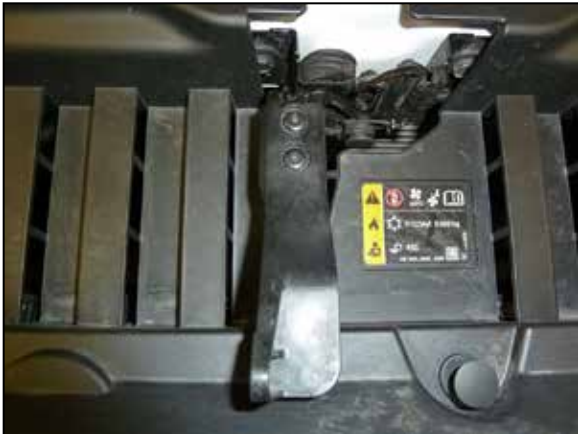
26. Reinstall the hood release arm and secure with the factory hardware.
