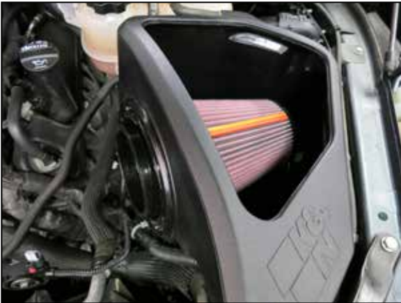
19. Install the air filter into the K&N airbox.
