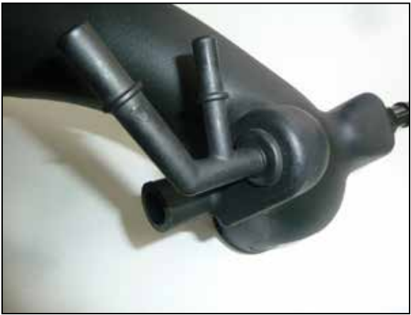
23. Install the provided ejector fitting into the K&N intake tube using the provided grommet.
