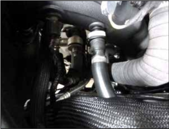
29. On 2WD models, cut one of the provided vent hoses to 11.5" long, install the two provided straight quick connect couplers and secure with the provided hose clamps. 4WD models skip to step #31.
