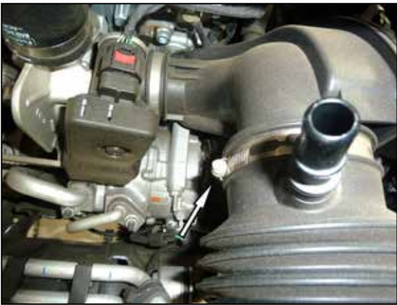
4. Loosen the hose clamp that secures the factory intake tube to the filter housing flex coupler.
