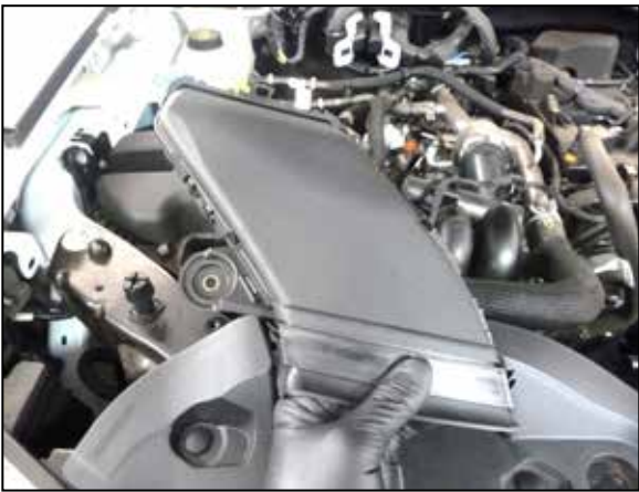
6. Lift the fresh air duct up and remove it from the vehicle.
