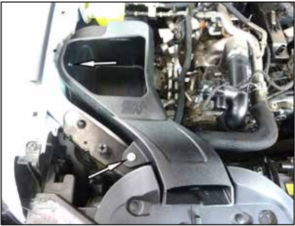
17. Install the K&N air filter housing into the vehicle so the mounting stud inserts into the factory grommet then secure the air box with the factory mounting bolts previously removed.
