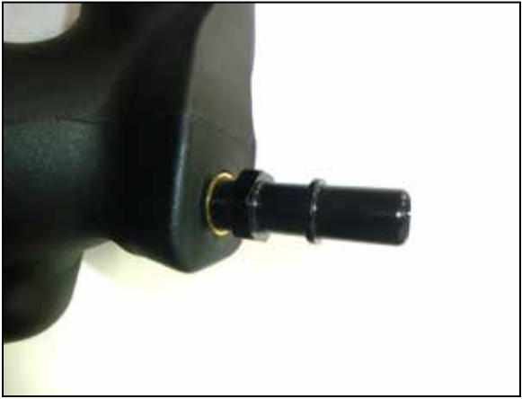
22. Install the provided quick connect fitting into the K&N intake tube as shown.
