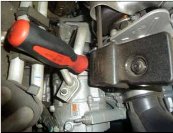
10. Loosen the hose clamp that secures the factory intake tube to the turbo inlet.
