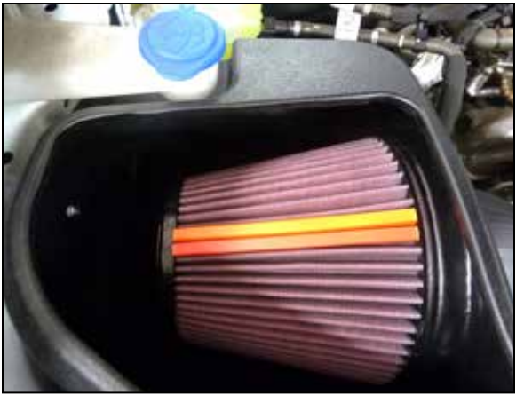
21. Install the K&N air filter into the air filter housing.
