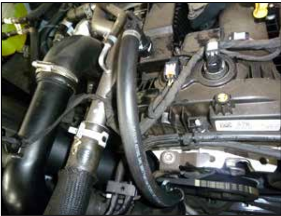
35. Connect the CCV hose assembly onto the CCV fittings on the engine and intake tube.
