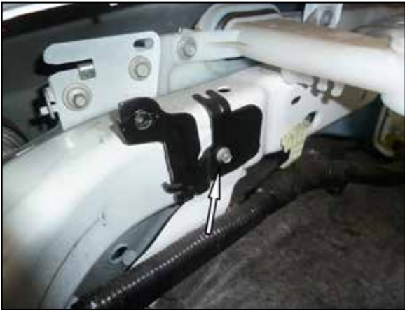
14. Remove the bolt that secures the air filter housing mounting bracket to the inner fender and remove the bracket from the vehicle.
