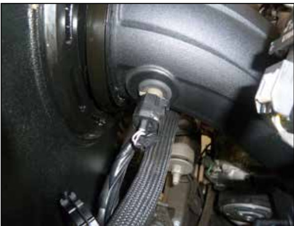
28. Reconnect the IAT sensor electrical connection.
