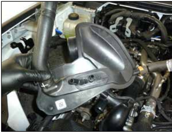
13. Remove the factory intake tube assembly.
