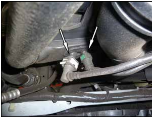
12. Release the locks and disconnect the ejector fitting hose connections.
