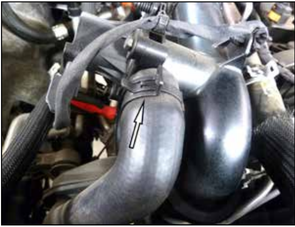
11. Release the spring clip that secures the BOV hose to the BOV valve and then disconnect the BOV hose from the valve.
