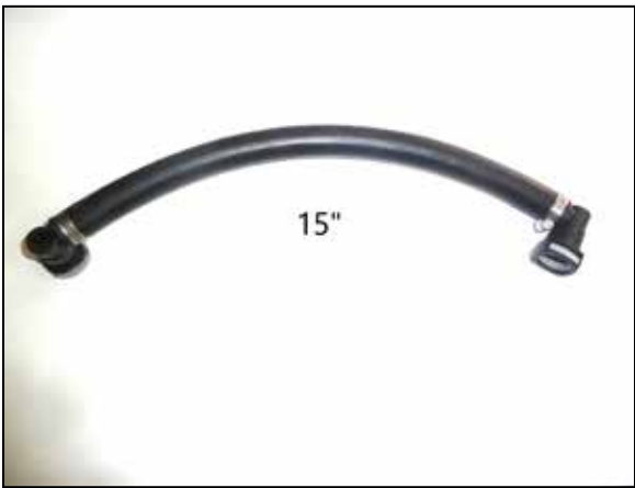
34. Install the two 90degree quick connect fittings into the provided CCV hose and secure with the provided hose clamps.
