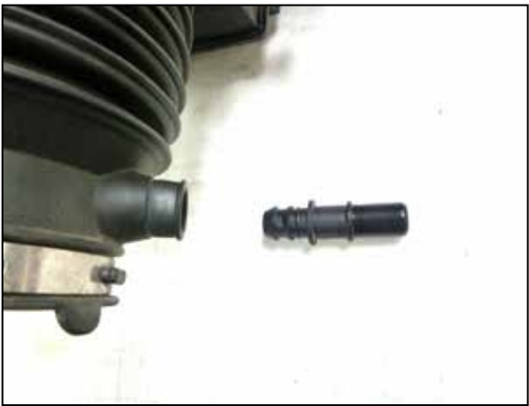
25. On 2wd models, remove the vent fitting from the factory intake boot.
