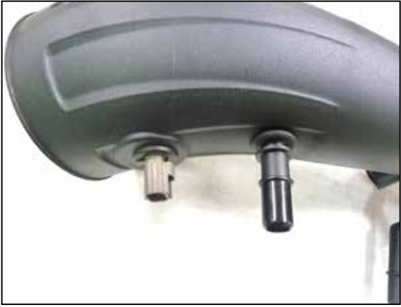
26. On 2WD models, measure 3.0" from the center of the IAT sensor and drill a 7/8" id hole. Be sure to remove any debris or shavings after drilling. Install the vent fitting into the 7/8" id hole drilled into the K&N intake tube using the provided larger grommet.
