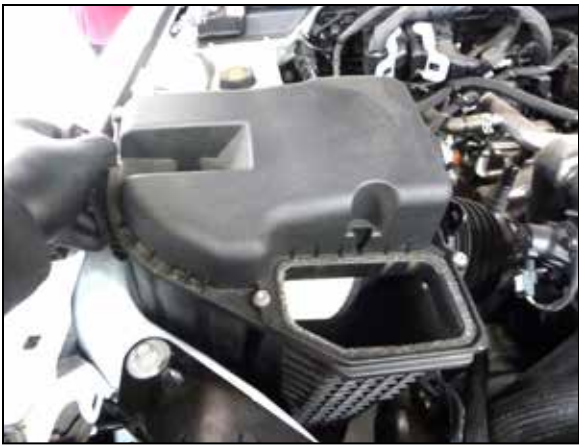
9. Remove the factory air filter housing from the vehicle.
