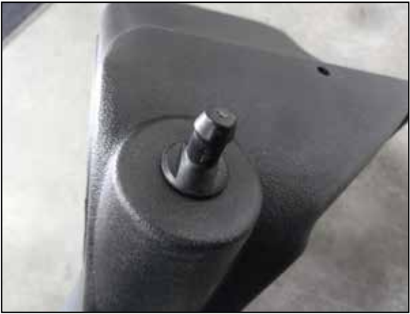
16. Install the provided mounting stud onto the K&N air filter housing using the provided hardware.
