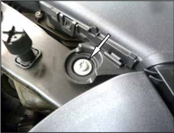
5. Remove the bolt that secures the factory fresh air duct to the core support. NOTE: This bolt will be reused.
