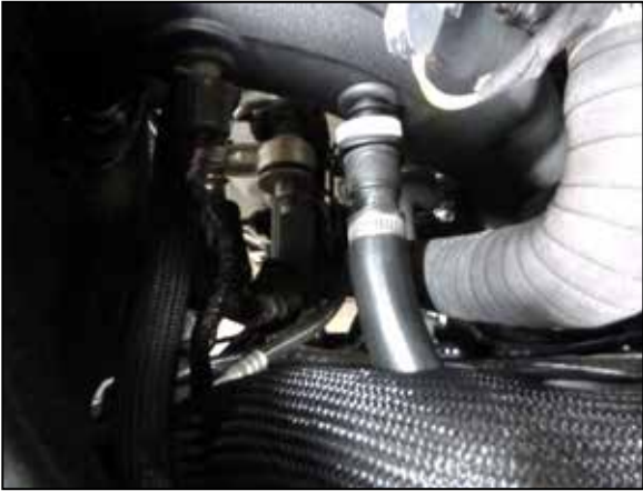
30. On 2WD models, connect one end of the assembled hose to the factory quick connect fitting installed into the K&N intake tube. Then connect the other end to the quick connect hose above the radiator.
