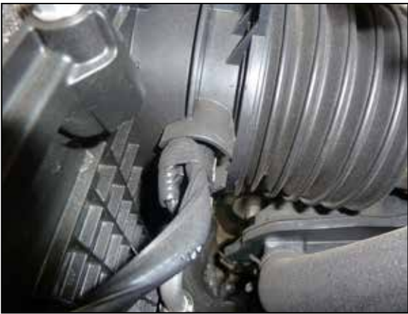
7. Disconnect the IAT sensor electrical connection.
