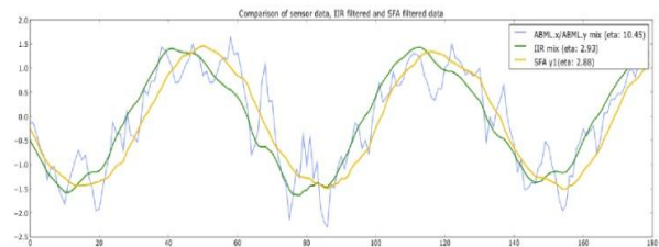
Figure 2. Comparing a weighted sum of the coronal acceleration sensors located at the shoulders to an IIR filtered signal and the slowest component extracted by SFA.
