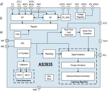
The external antenna is directly connected to the Analog Front-end (AFE), which amplifies and demodulates the received signal. The watchdog continuously monitors the output of the AFE and alerts the integrated lightning algorithm block in the event of an incoming signal. The lightning algorithm consists of hardwired logic.
