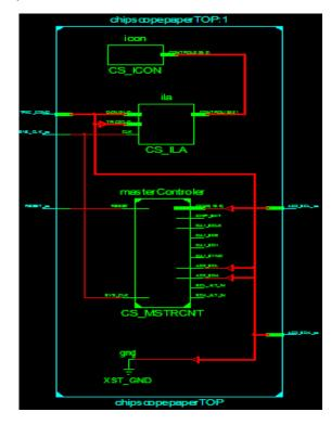
Figure 4. Internal view of Register Transfer Tevel (RTL) Synthesis result showing interconnection of "masterControler", "icon", "ila" modules within the top level entity "chipscopepaperTOP".
