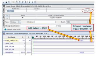
Figure 6. Xilinx ChipScope-Pro Logic Analyzer showing Field Programmable Gate Array (FPGA) internal signal; pertaining to the output of ADC, its driving signals and external hardware conditional trigger input in run-time.
