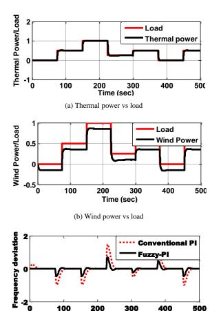
Time (sec) (c) Frequency deviation. Fig. 5 Power and frequency variations in the hybrid system for step change in load demand.
