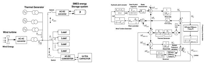
Fig.1 Block diagram of the hybrid distributed generation system (a) system integration (b) system transfer functions.
