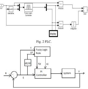
Fig. 3 Block diagram of a fuzzy based PI controller.
