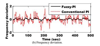
Fig. 6 Frequency variations in the hybrid system for random change in wind speed.
