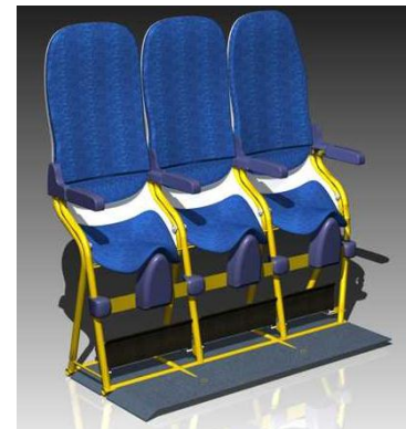
Figure 2. SkyRider Vertical Seat Design Concept [9]
