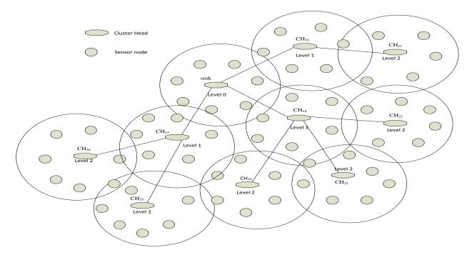
Figure 1. Cluster heads arranged as multilevel tree.
