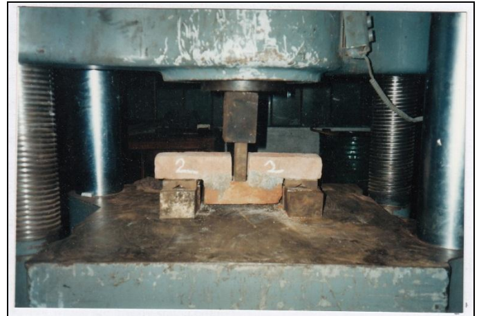
Figure 4. Mortar tensile test setup
