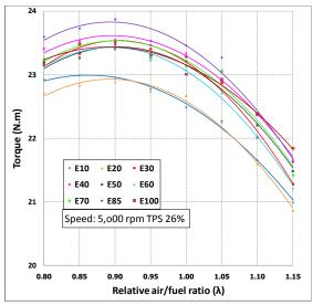
Figure 4. Variation of break torque with air-fuel ratio
