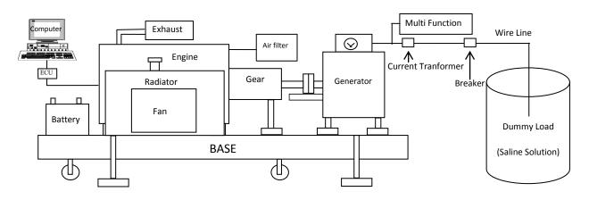
Figure 1. Schematic view of the experimental setup.
