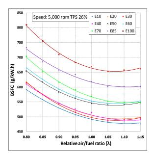
Figure 5. Variation of BSFC with air-fuel ratio
