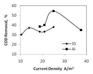
Figure 2: COD removal at different current densities
