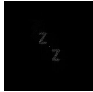
Figure2. The image reconstructed by using SHSP method from the hologram in Fig. 1(b)
