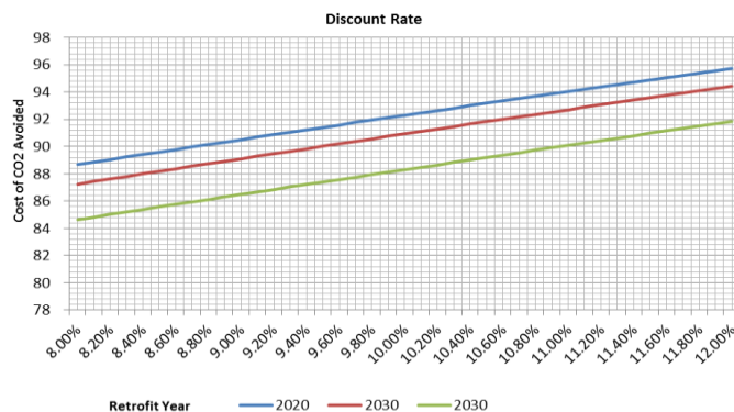
Figure 3 The estimated cost of CO 2 avoided for retrofitting the underlying CCGT plant to 90% CO 2 capture (in USD)
