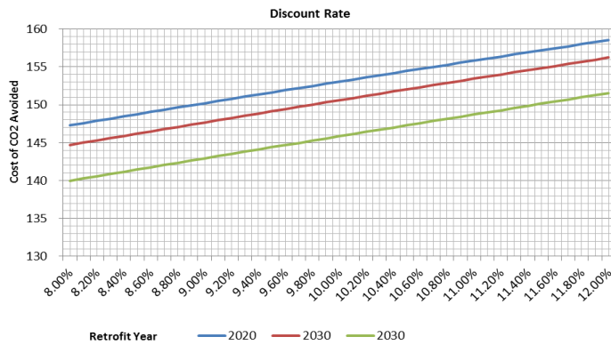
Figure 5 The estimated cost of CO2 avoided for retrofitting the underlying CCGT plant to 50% CO2 capture (in USD)
