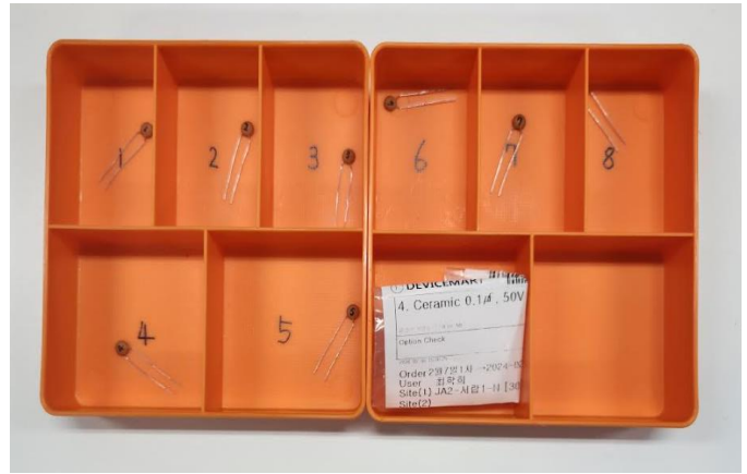
Figure 7. Measured Capacitor Samples
