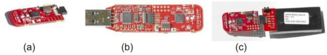
Figure 3 ZNP Mini Kit [9] (a) ZNP Mini Kit Target board, (b) eZ430 USB Stick with target board (c) ZNP Mini Kit Battery board
