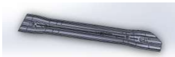
Fig.1 CAD model of Anti-intrusion bar
