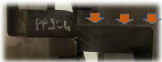
Fig.7 Deformation of the PP TPC material during the shear test.
