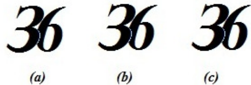
Figure 8: Selective attention . (a) An input pattern. (b) The recognizer gradually reinforces pixels that corresponds to objects in its template library, and inhabits those that do not, yielding a partial recognition. (c) After a delay, attention is switched to unmatched regions, and another match to the library is found (after Fukushima).
