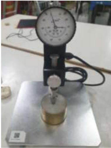
Figure 3. Fall Cone Penetrometer
