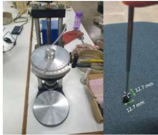
Figure 2. Laboratory Miniature Vane Shear
