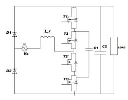
Figure 3. Power circuit of a unidirectional three level flying capacitor converter.
