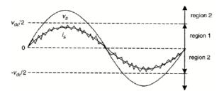
Figure 7. Operating regions of a three level converter.
