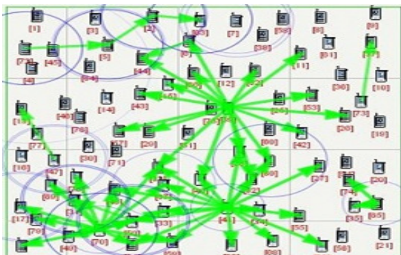
Figure 2. Second network scenario comprising of randomly deployed 80 nodes with 8 different source destination pairs.
