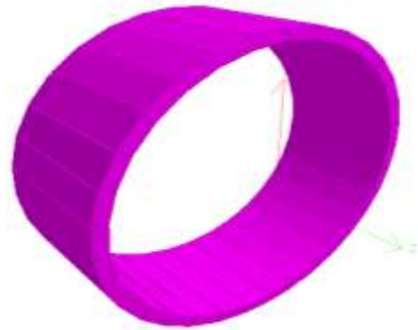
Fig. 5 Final tunnel lining model
