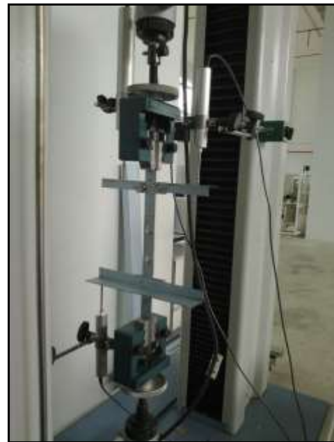
Figure 4. Single shear connection test setup
