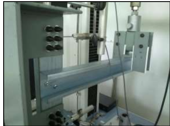
Figure 7. Moment Connection Test Setup
