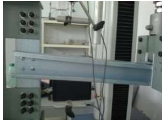
Figure 12. No buckling failure (BC4)
