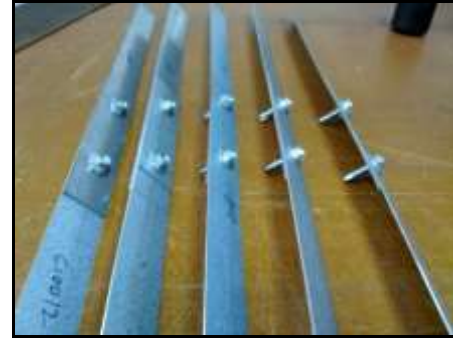
Figure 3. Tensile test specimens
