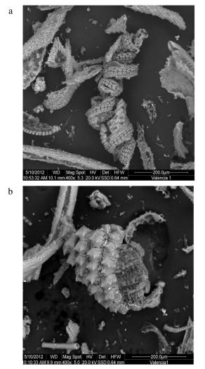
Figure 2: ESEM for two different zones of ash samples The chemical analysis was applied for some spots in images of larger magnifications, as shown in Figure 3. ESEM inspection and the chemical analysis for some spots showed that the straw ash samples are consisting primarily of silica, high amounts of chlorine, potassium and observed amounts of other elements such as Ca and Mg at the selected spots, similar results have been found by Said et al. [10].
