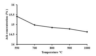
Figure 1: Ash concentrations at different temperatures.
