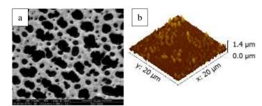
Figure 1. Morphology of zinc oxide scaffolds recorded by (a) SEM and using AFM in non-contact mode.
