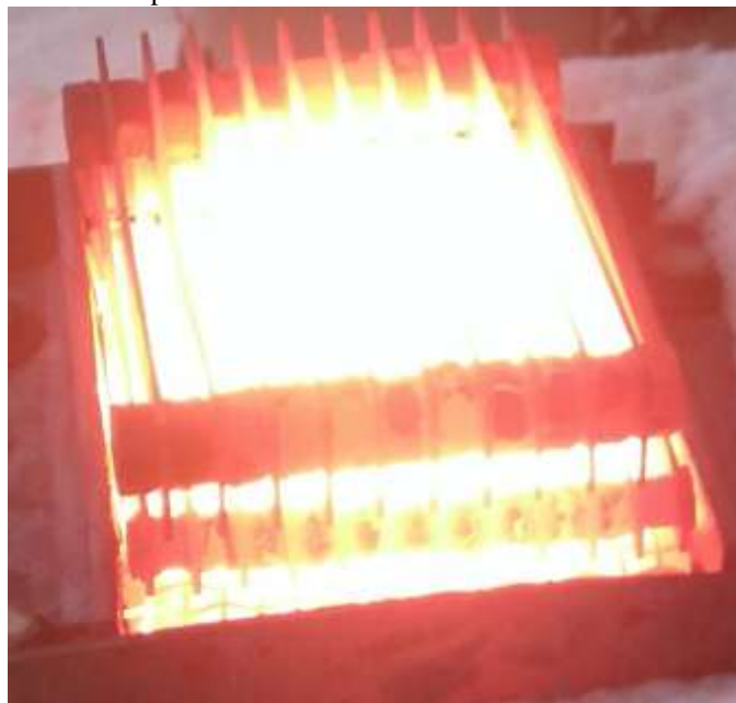
Fig. 1. A photo of the infrared burner operating without a permeable matrix in the mode of stimulated surface combustion near the surface of the recuperative elements. Combustion intensity 290 W/cm 2 , air ratio is equal 1.4.
