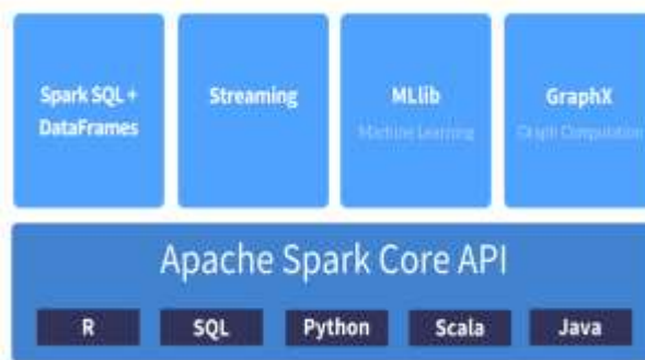
Figure 3. Apache Spark architecture
