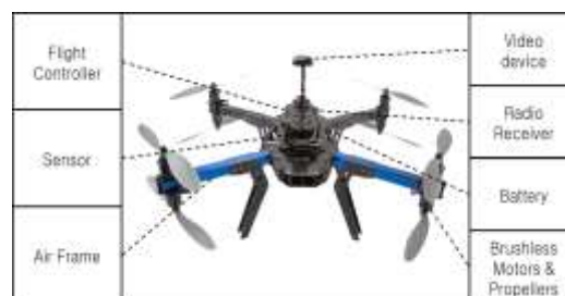
Figure 1. Drone's basic structure
