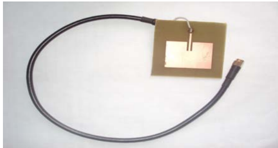
Figure 11. Fabricated RMSA with Inset Line Feed
