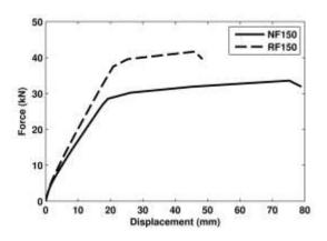
Figure 5. Predicted displacement-force relationship of flexural critical beams
