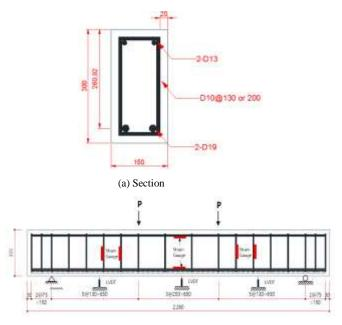
(b) Test setup for shear critical beam (RS150-S1)
