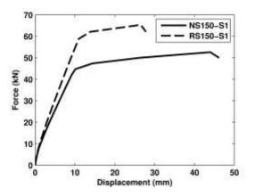
Figure 4. Predicted displacement-force relationship of shear critical beams
