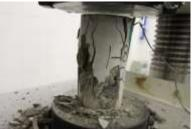
Figure 7. Compressive test of concrete with 3D fiber
