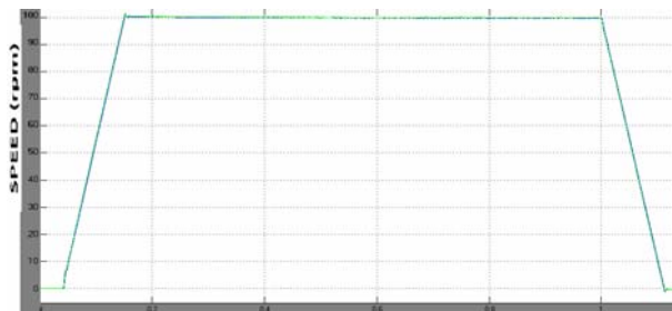
Fig. 5a actual speed and reference speed for 100 rpm.
