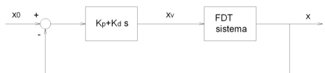
Figure 13. System control scheme
