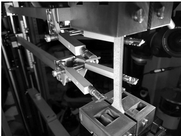
Figure 6. Tensile strength test on 3D printed specimens.
