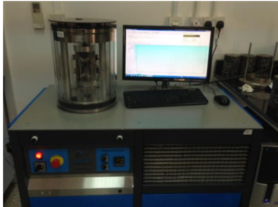
Figure 5. AMPT system for dynamic modulus test
