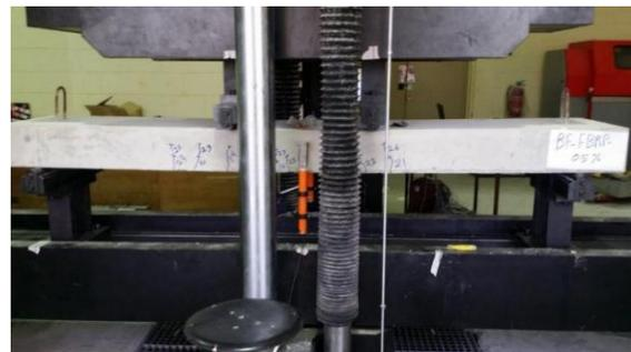
Figure 6 One-Way Concrete Slab during Flexural Test.
