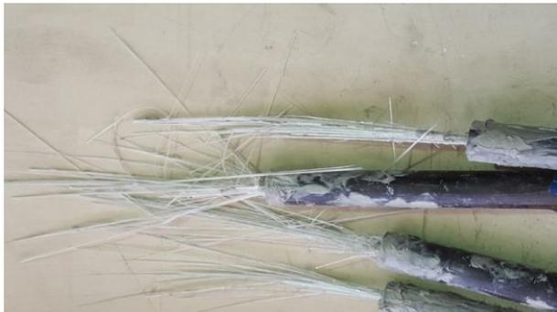
Figure 4. GFRP Reinforcing Bars after Failure.
