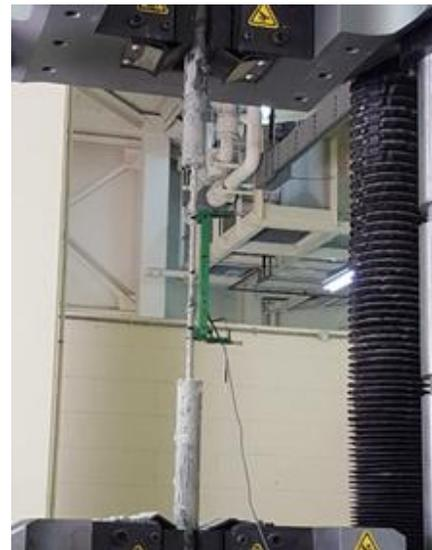
Figure 2. FRP Reinforcing Bar under Tensile Strength Test.
