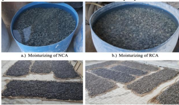
Figure 1: Moisturizing and Drying of Aggregates.
