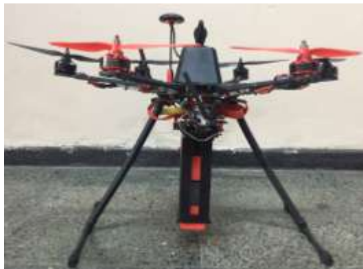
Figure 2. Front view of realized LTS on hexacopter.
