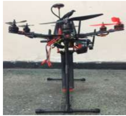
Figure 3. Side view of realized LTS on hexacopter.
