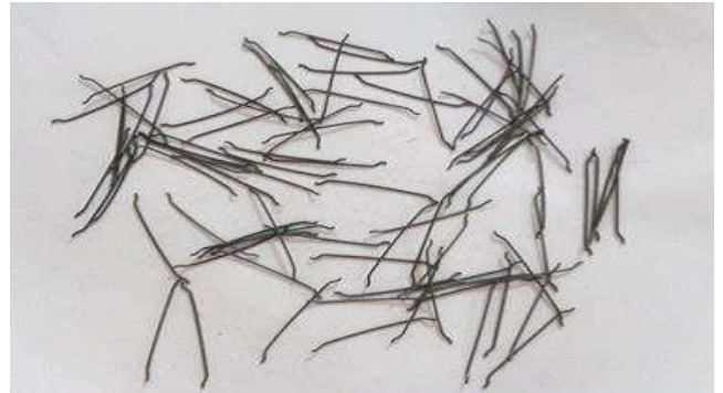
Figure 3. Hooked end steel fibres of aspect ratio 50
