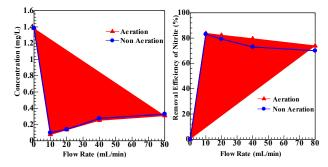
Figure 4. NO<sub>2</sub>-N removal concentration and efficiency of noodles wastewater after treated with aeration and non aeration MSL system
