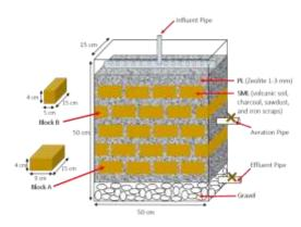
Figure 1. Design of MSL system [9].
