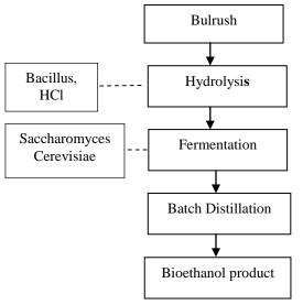
Figure 1. Bioethanol production flow used hydrolysis process, fermentation process, and batch distillation
