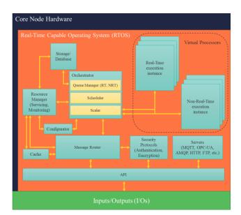
Figure 5. Proposed Software Architecture of Core Node.
