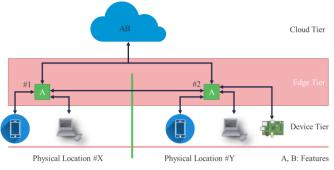
Figure 3. Simplified topology of the Edge Computing network.
