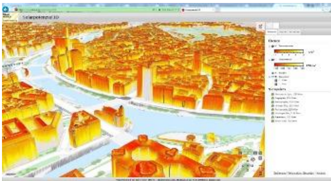
Figure 4. “LASERDATA” one of the Solar Potential Analysis applications that could help policy makers to estimate the energy yield of photovoltaic installations and plants, to evaluate the solar heating and cooling of buildings or to plan the positioning of solar thermal or photovoltaic modules. https://www.laserdata.at/services.html
