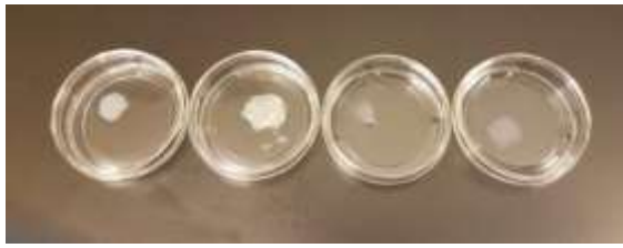
Figure 6 3D printed samples showing hydrogel constructs including 3T3 cells in media after 7 days using different bioinks. From left to right, IK6 15 mg, IK6 20 mg, Biogelx™ 20 mg, Biogelx™ 40 mg.
