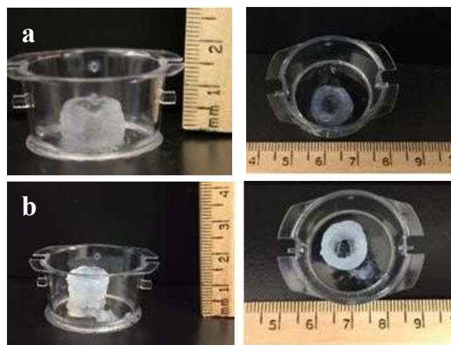
Figure 3 3D printed constructs (a) A 9 mm height construct was printed using Biogelx™ 40 mg/mL with our robotic 3D bioprinter and a 3D printed construct of 15 mm height was printed using 20 mg/mL IK6 with our robotic 3D bioprinter (b)
