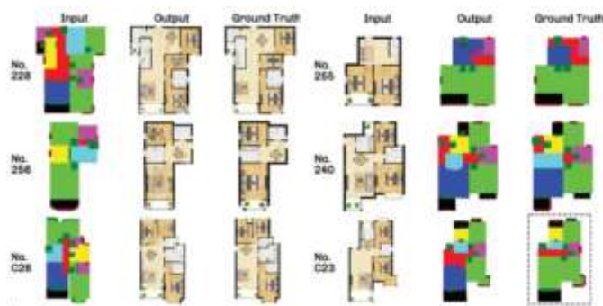
Left: color labeled map input, output of functional floor plan and actual floor plan
