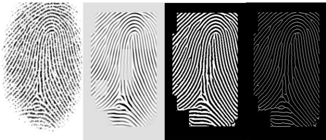
Figure 4: (a) Original Image, (b) Enhanced Image, (c) Binarised Image, (d) Thinned Image
