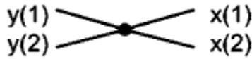
Fig. 1. Radix-2 butterfly representation showing the dependence between two inputs and two outputs.
