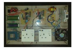
Figure 3. RFID electrical power meter for testing.
