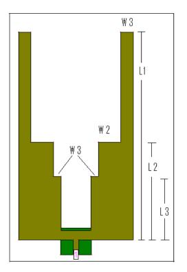
Figure 1: Structure of Proposed antenna.
